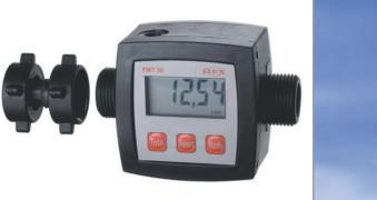
The FMT 50 PP uses an interlocked impeller in the measuring chamber which guarantees fast and safe filling. Suitable for use with low viscosity liquids in conjunction with our JUNIORFLUX & COMBIFLUX pumps, as well as in fixed installations. (Not suitable for use with flammable liquids)
