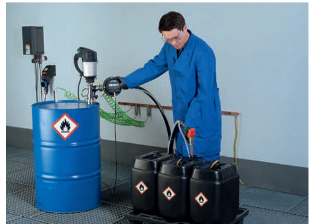
Semi-automatic can filling in explosion zone 1.
